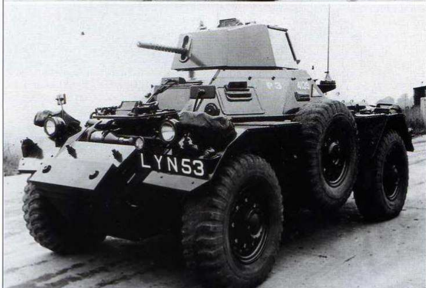
Prototype number 3 photographed after the hull has been raised by the addition of a welded strip. This may be the same vehicle as shown in its original form (see page 16), but it has been registered LYN 53, and now carries its full complement of accessories. Note how the engine-compartment covers have been welded together in pairs.
