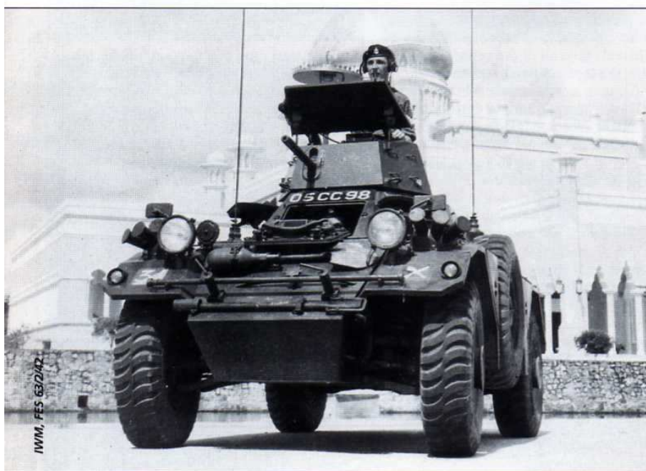
The Mk 2/2 was modified in the field by the inclusion of a fixed collar between the hull and the turret.
