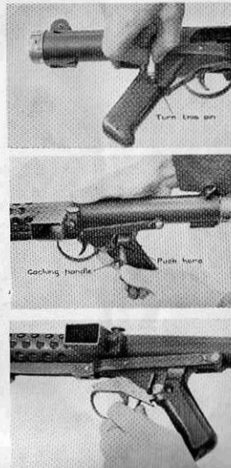
Fig 4.—Taking out the trigger group
