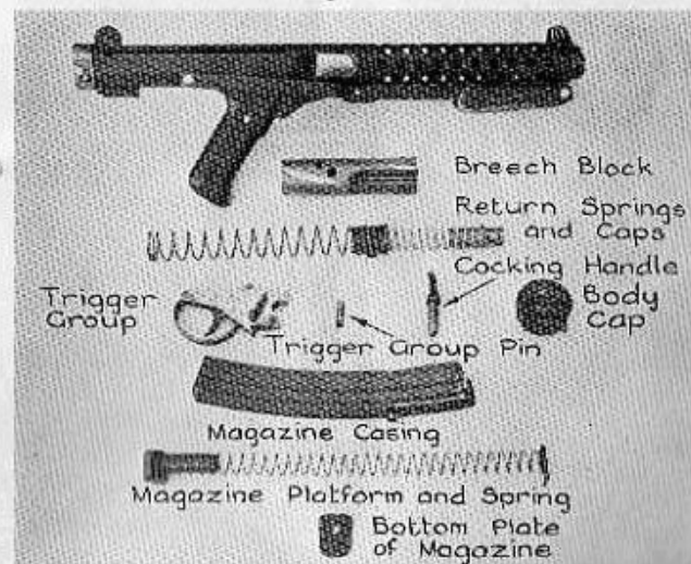
Fig 1 (b).—The Sub Machine Gun, L2A2 (components)
