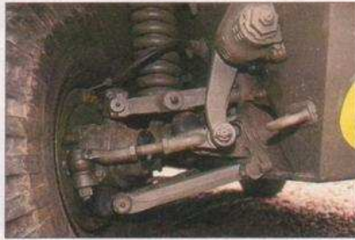
The suspension arrangement is the key to the Ferret's cross-country ability - it has an exceptionally long travel. As this view shows, it's also pretty indestructable.
