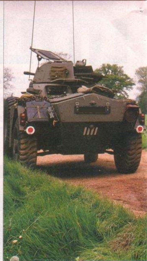
The suspension arrangement is the key to the Ferret's cross-country ability - it has an exceptionally long travel. As this view shows, it's also pretty indestructable.
