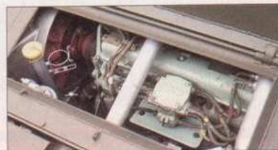
Power is provided by a Rolls Royce B60 engine (which is NOT the same as the FB60 fitted to the Vanden Plas 4 litre R, although the two are related). Notice the enclosed distributor and HT leads - Ferrets can "wade" in up to 3ft of water without any special preparation.
