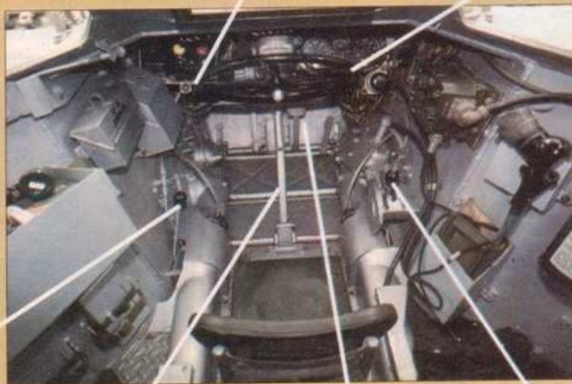
Power is provided by a Rolls Royce B60 engine (which is NOT the same as the FB60 fitted to the Vanden Plas 4 litre R, although the two are related). Notice the enclosed distributor and HT leads - Ferrets can "wade" in up to 3ft of water without any special preparation.
