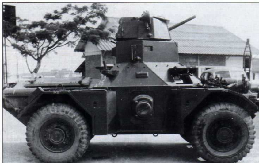
The Mk 2/2 was modified in the field by the inclusion of a fixed collar between the hull and the turret.
